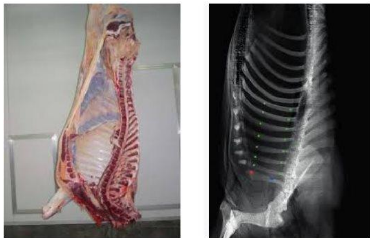
Figure 15: X-ray imaging-based 3D vision capability is being developed for Robot butcher.
