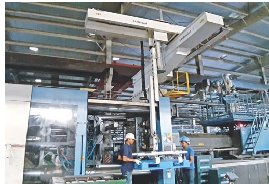
Figure 21: Robots are being used in loading and unloading
