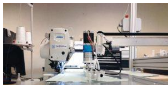
Figure 19: Robots with the capability of handling fabrics and performing sewing
