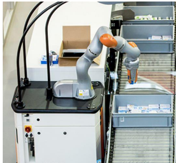
Figure 14: Robots with stereo vision are in operation of picking objects
