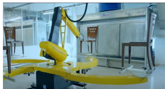
Figure 22: Robots are in action in finishing furniture in local factory.
